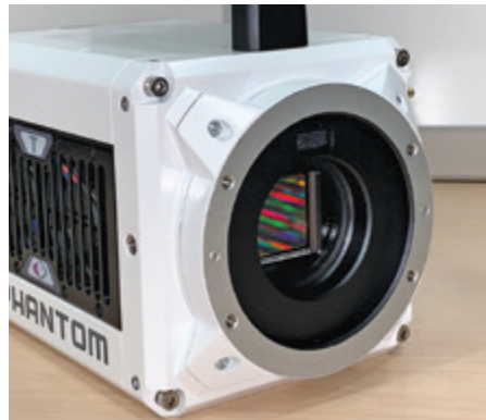
Front with F-mount removed
