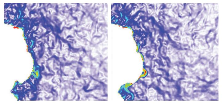
The high-speed footage also showed how effective masks are at minimizing variations in airflow—and therefore the spread of gases.
