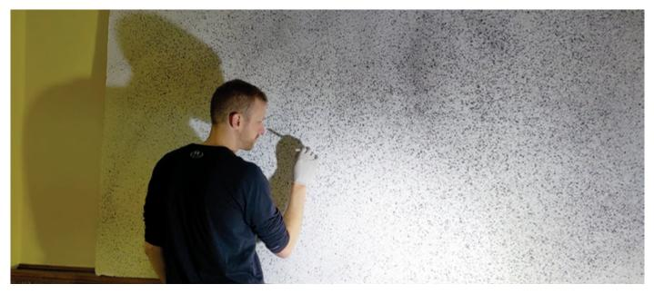
A black marker is being used make small dots in places on the drywall with relatively low speckle areal density. The image of these speckles by the camera are what become distorted by slight changes in the air, revealing the air flow that can be imaged using a high-speed camera.
